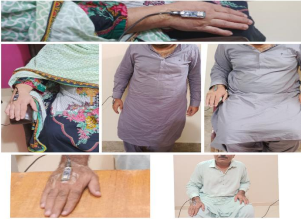
Figure 02: Subjects wearing IMU sensor to show the different hand resting position
