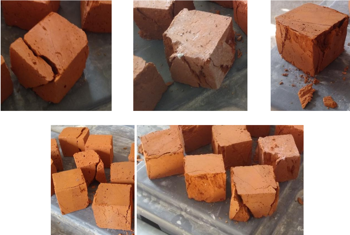
Figure 4.3. The failure shapes of bricks
