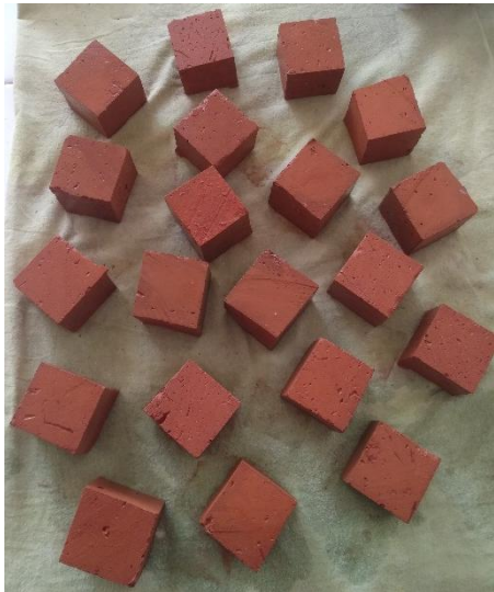
Figure 4.1. Clay bricks cut in size 50×50×50 mm
