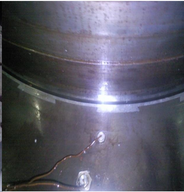
Figure 2. Turbine guide bearing white metal.
