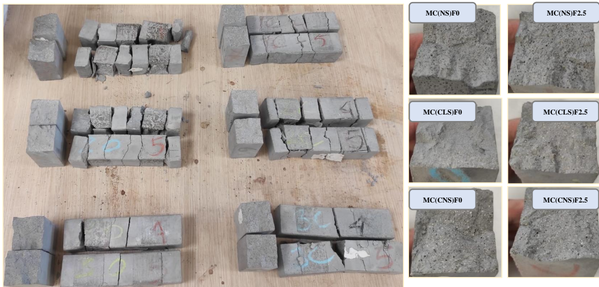
Figure 4. General view of the specimen after flexural tensile and compressive strength tests
