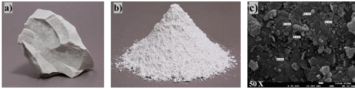
Figure 2.1. Different form of Bentonite clay, a) rock, b) powder, c) nano particle (Esan)
