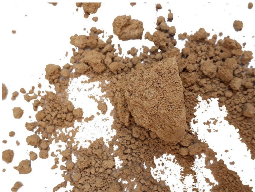
Figure 3.1. In the composite prepared with 70% NSP and 30% PR, fragmentation of the sample occurred due to the insufficient amount of matrix and the inability to obtain homogeneous mixtures
