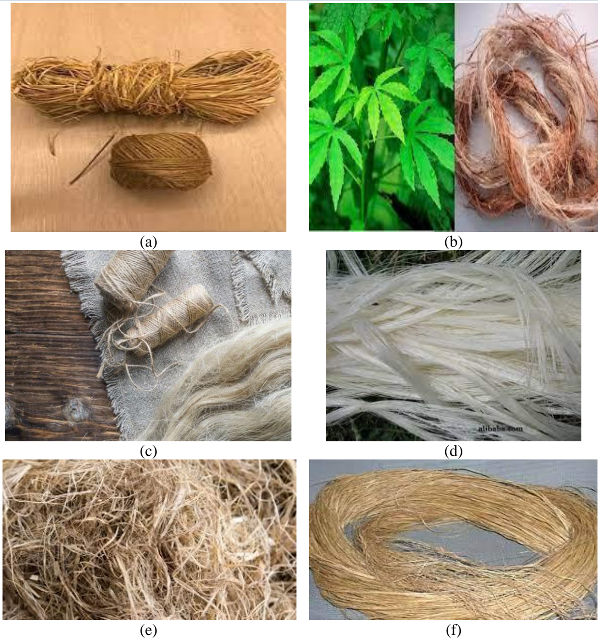
Fig. 2.1. Well-known bast fibers in the literature a) Jute, b) Kenaf, c) Flax, d) Sisal, e) Hemp, f) Ramie
