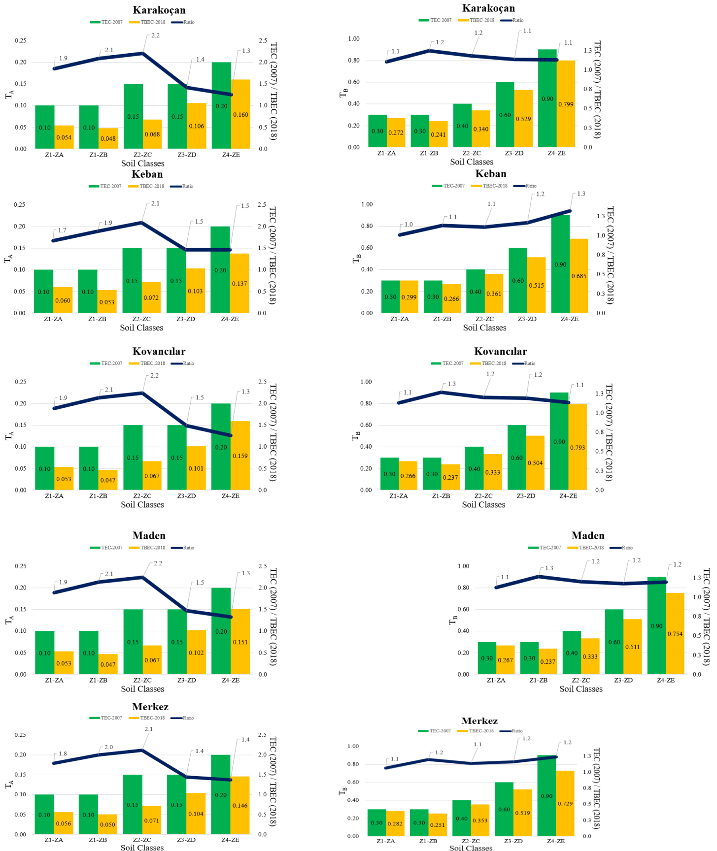
Figure 3.3. Comparison of corner periods for Karakoçan, Keban, Kovancılar, Maden and Merkez districts
